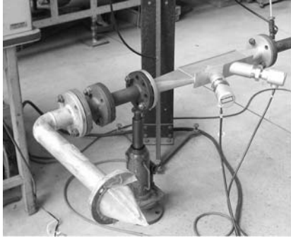
Case 2 (5D straight pipe + horizontal elbow)
